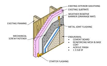
Fig. 6.1 – Standard Wall with Rigid Insulation
