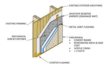
Fig. 6 - Standard Wall Construction
