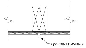
Fig. 5 - Vertical Panel Joint
