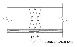
Fig 5.1 – Caulk Joint w/ Bond Breaker Tape
