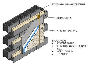
Fig. 6.3 – Block Wall with Furring
