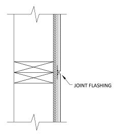
Fig. 8 – Horizontal Panel Joint Spacing
