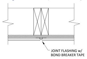
Fig. 5.2 – Flashed Joint w/ Bond Breaker Tape
